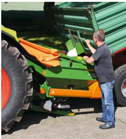
Filling with tipping trailer
